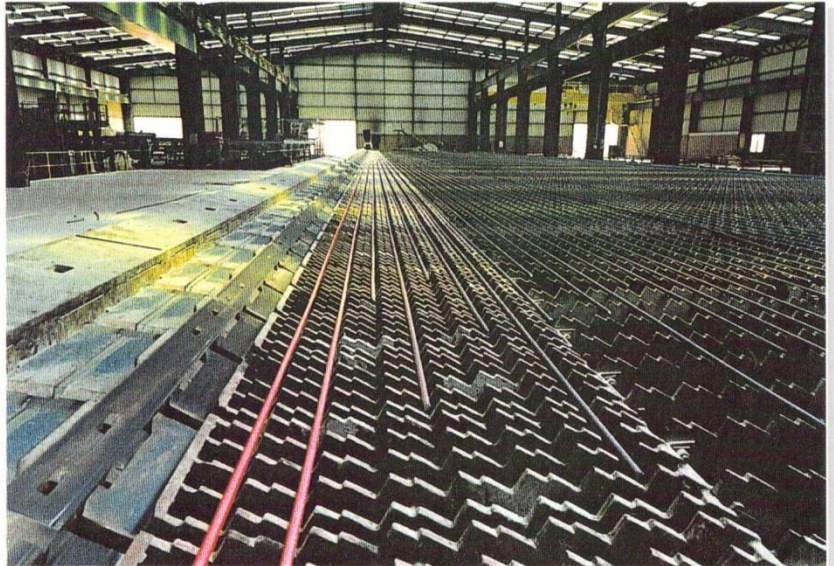
Rechenkühlbett Rake type cooling bed
